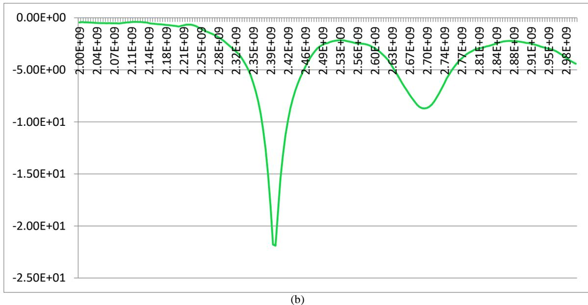
Figure 5. (a, b): ( $S_{11}$ ) measurements result of the antenna fed via coaxial probe ( BW = 52.4 MHz)
