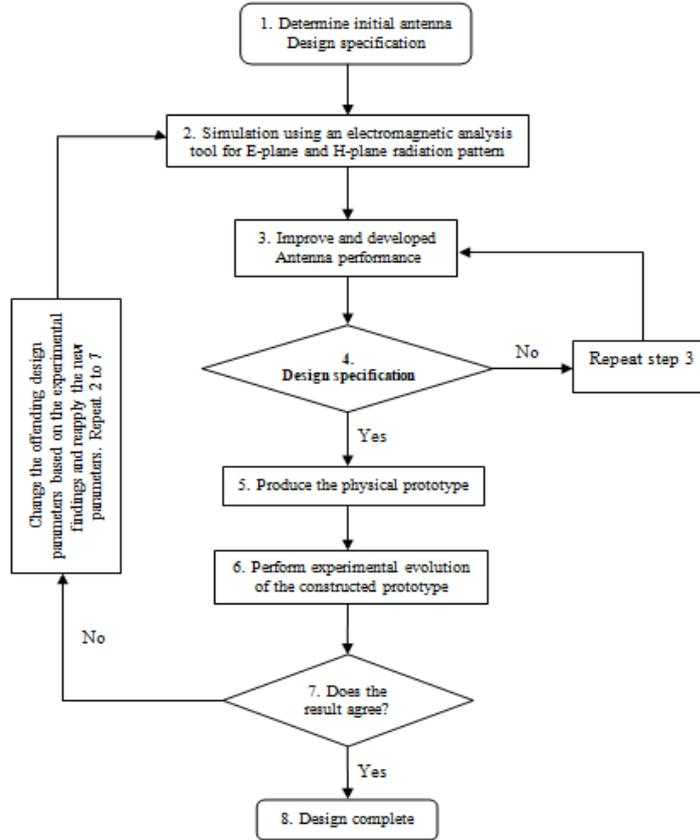
Figure. 1. Antenna Design and Development Flow Chart
