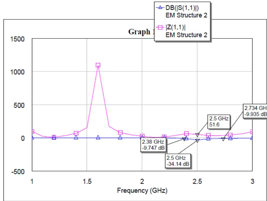
Figure 6. Simulated Input Impedance  $Z_{in}$
