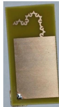
(b). Antenna prototype (fabricated)
