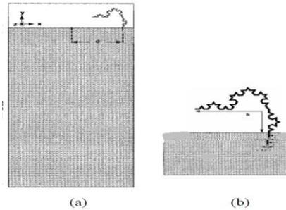
Figure.3 (a & b). The dimensions of the folded Koch curve monopole fed via coaxial probe
